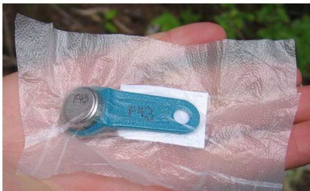
Figure 1. An iButton (Maxim DS1922L) wrapped in plastic wrap, ready to be buried in the ground below a tree.
