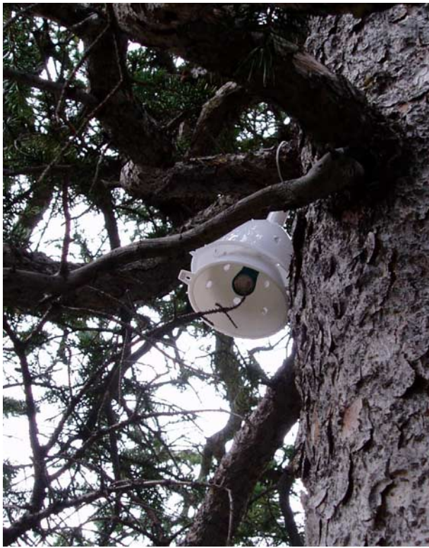
Figure 1. An iButton in a funnel radiation shield in a tree.
