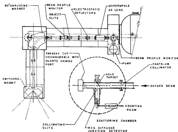
FIG. 1. External beam system of University of Washington FN tandem Van de Graaff accelerator showing position of scattering chamber.
