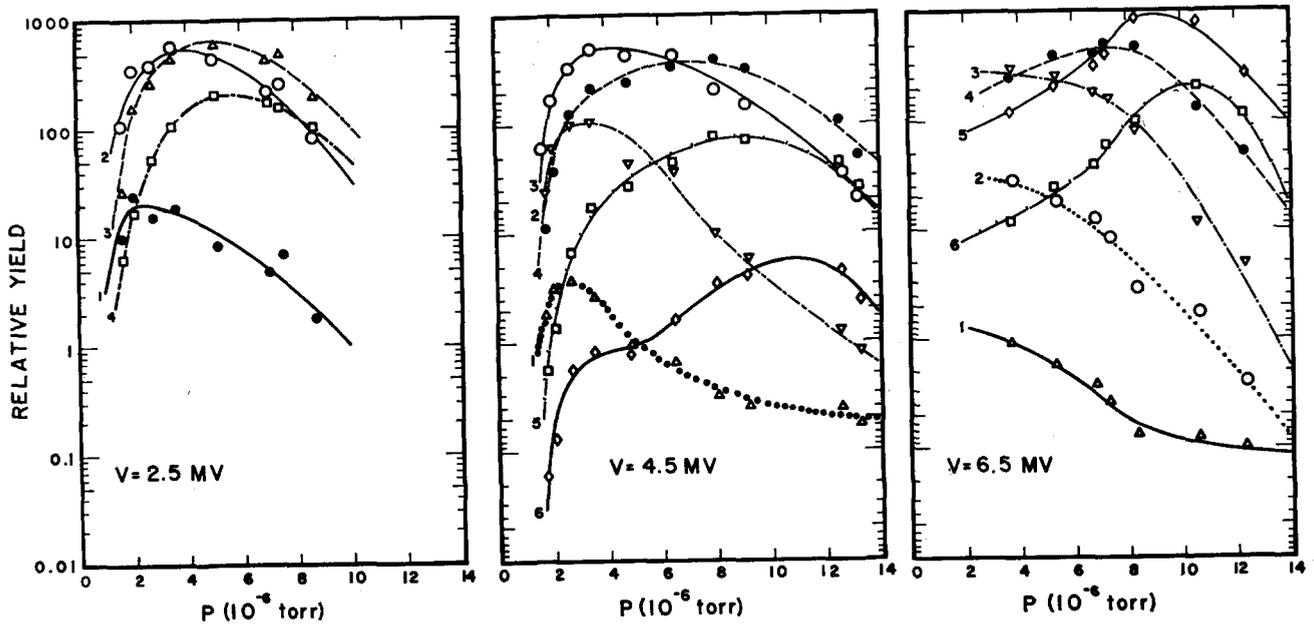
FIG. 3. Observed yield of multiply charged ions as measured with apparatus shown in Fig. 1 over a range of stripper pressures at three terminal potentials. The small numerals at the left end of the curves indicate the charge of the ions.
