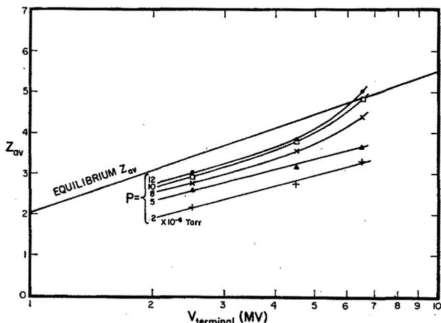
FIG. 4. Average charge computed from measurements shown in Fig. 3 as a function of terminal potential and stripper pressure. Calculated average equilibrium charge is shown for comparison.
