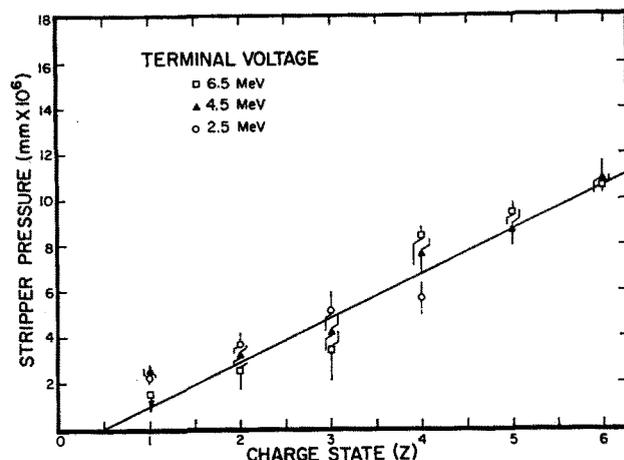
FIG. 5. Optimum stripper pressure to give maximum yield of a particular charge state at three terminal potentials. Flags indicate pressure range over which 90% of maximum yield is maintained.
