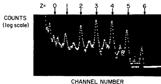
FIG. 2. Pulse height spectrum observed with 6.5 mV terminal potential. Arrows indicate positions of charge state peaks.
