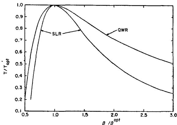
Fig. 2. Transit time factor versus velocity ratio for two types of resonant accelerator cavities. SLR is the 3-gap split loop resonator of Stony Brook type; QWR is the 2-gap quarter wave resonator of Stony Brook/Weizmann type. Both are calculated using an analytic expression [1] based on the sharp cutoff approximation.
