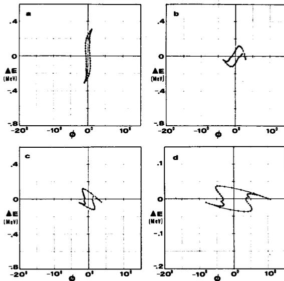
Fig. 4. Energy-phase plots calculated by program ENTIME for a  $^{40}\text{Ca}$  ( $15^+$ ) beam at four locations in the accelerator: (a) at linac entrance; (b) before 180° bend; (c) after 180° bend; and (d) debunched on target (note change in energy scale). Time scale (at 150 MHz) corresponds to 18.5 ps/degree.
