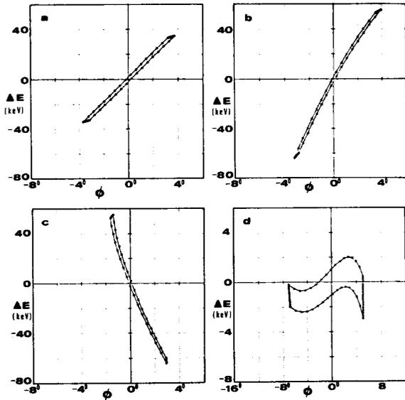
Fig. 3. Energy-phase plots calculated by program ENTIME for a proton beam at four locations in the accelerator: (a) at linac entrance; (b) before 180° bend; (c) after 180° bend; and (d) debunched on target (note change in phase and energy scales). Time scale (at 150 MHz) corresponds to 18.5 ps/degree.
