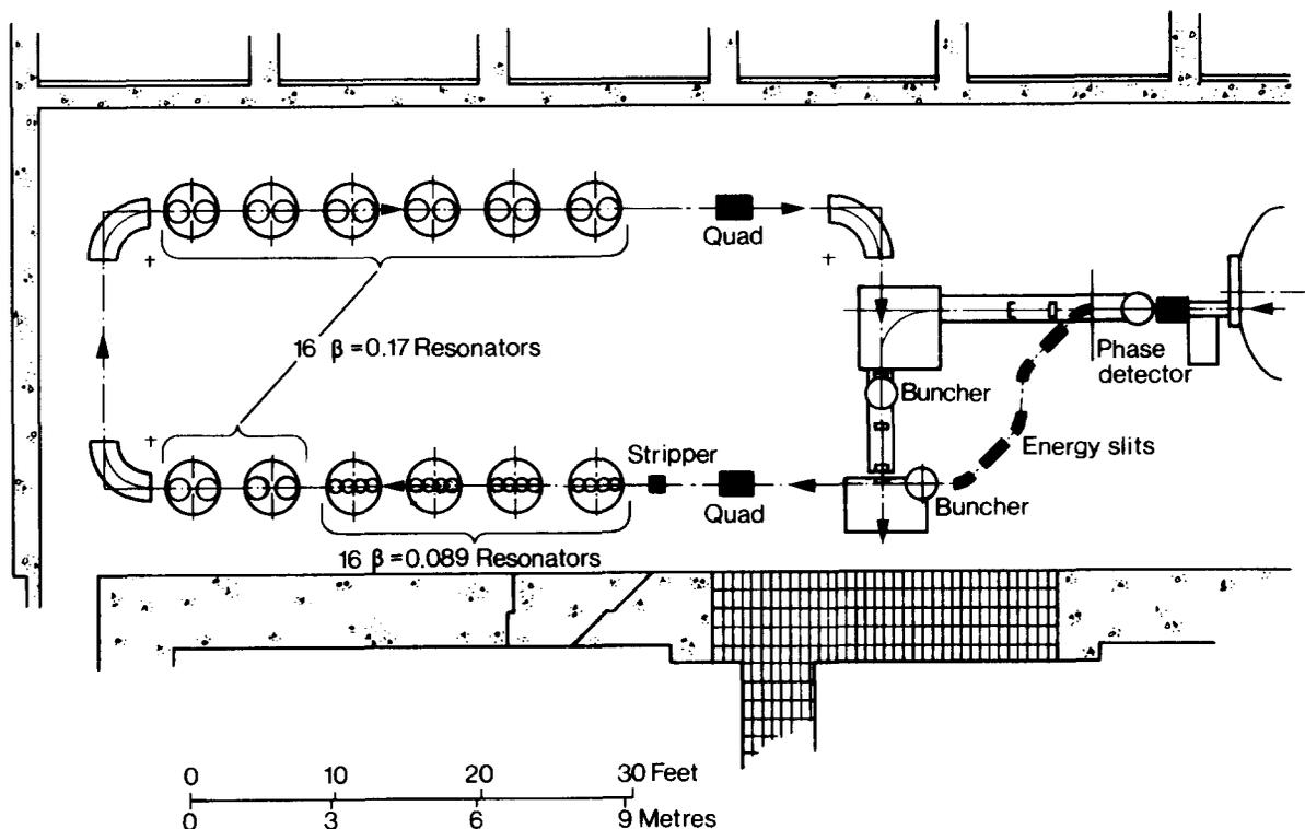
Fig. 1. Layout of UW NPL superconducting booster linac. Quadrupole doublet focusing elements (not shown) are placed between cryostats (circles) and between pair of  $90^\circ$  magnets at left of diagram.
