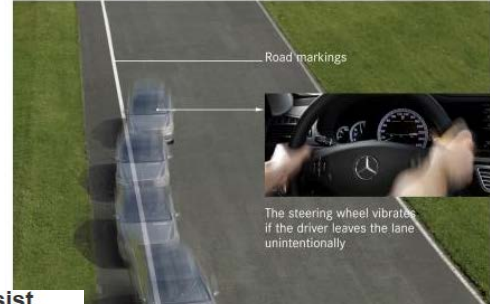
Lane-departure warning system: steering wheel vibrations warn the driver if he or she is veering out of the lane
