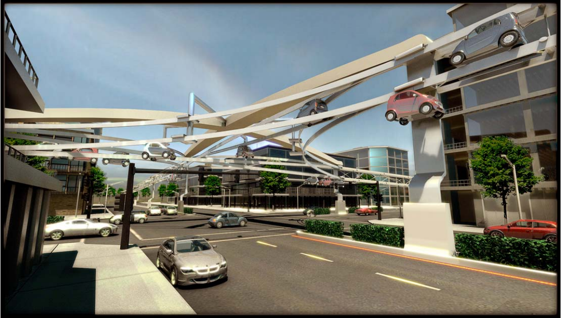
Figure 8 illustrates a full, high-capacity, 25 mph interchange above a common street intersection.
