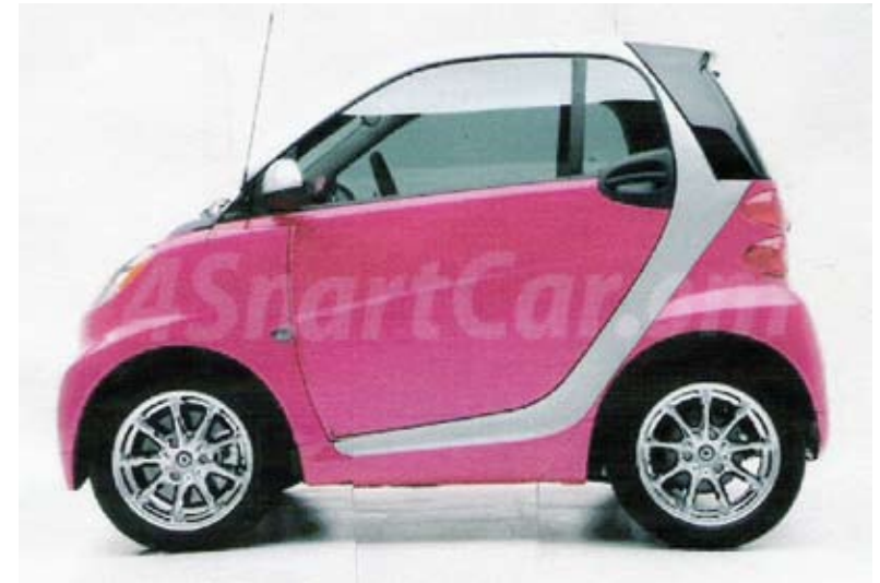
FIGURE 3-1 illustrates a slightly foreshortened Mercedes Benz Smart car montage-cropped to have a wheel base and overall length as proposed for the Rail Car. As shown the auto is foreshortened 14".
