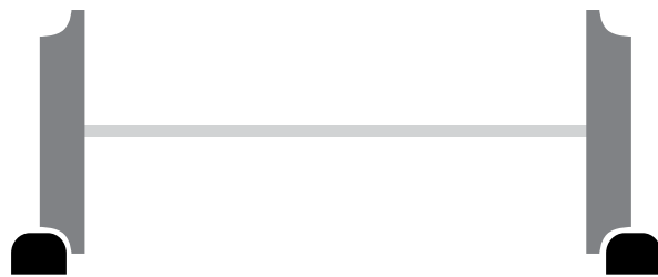
FIGURE 4-12 illustrates the capture of a railroad axle by means of two rails.
