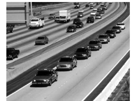
FIGURE 1-2. An experiment in platooning with lateral control and 6 meters of headway between cars at 60 mph.
