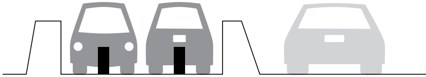
FIGURE 4-1 1D. Two-way traffic Rail traffic is illustrated within a single converted HOV commuter lane. The Rail is not elevated, needs no skeleton, and is protected with standard barriers.
