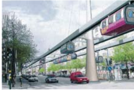
FIGURE 1-3E. Two way PRT transport down the centerline of a boulevard is illustrated using a modern suspension type bridge support.
