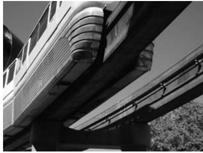
FIGURE 4-13A illustrates the 5 wheels of a single Doobie which constrain 3 degrees of freedom. FIGURE 4-13B is a photograph of a vehicle on Seattle's monorail secured by such Doobies to a concrete rail.
