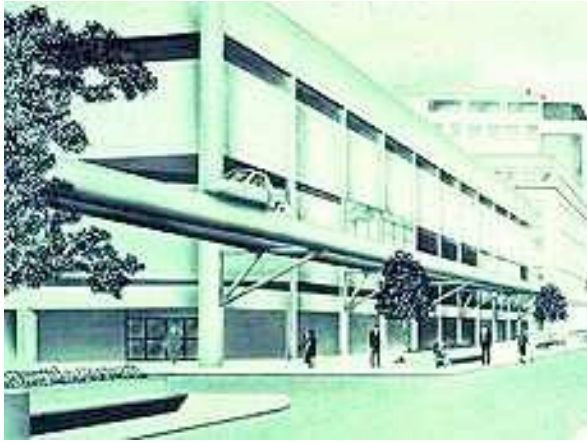
Figure 3.7. The guideway can be attached to facades
