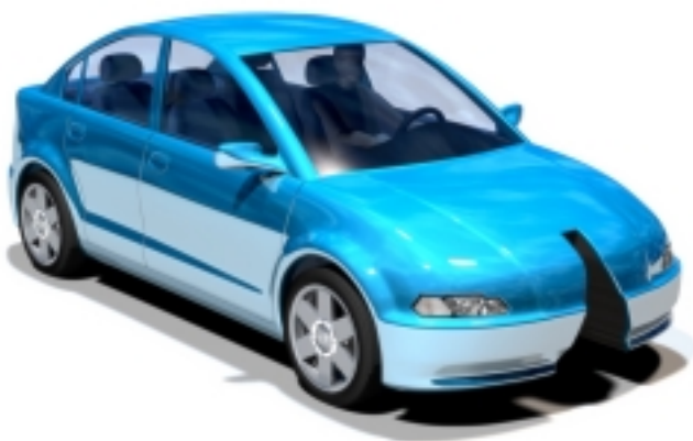
Figure 3.28. RUF electric car for road and guideway
