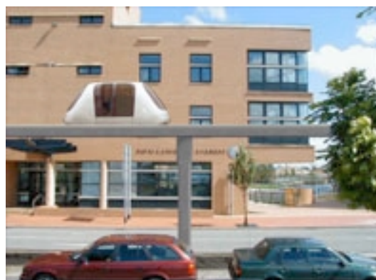
Figure 5.5. ULTra guideway for Cardiff
