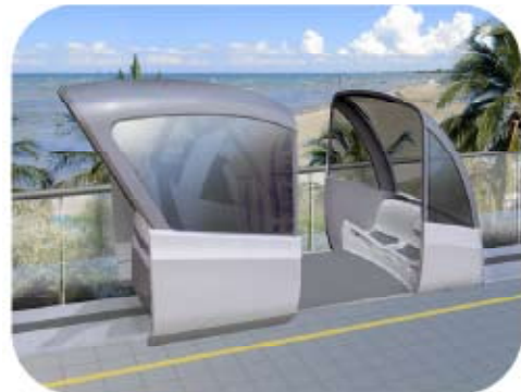
Figure 3.5-4: 3-Passenger Cabin with Open Door
