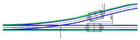
Figure A-9 - Switch Interchange Image Courtesy of Vectus
