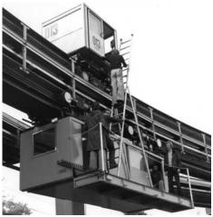
Figure 18 - Cabintaxi Emergency Evacuation Image Courtesy of Cabintaxi
