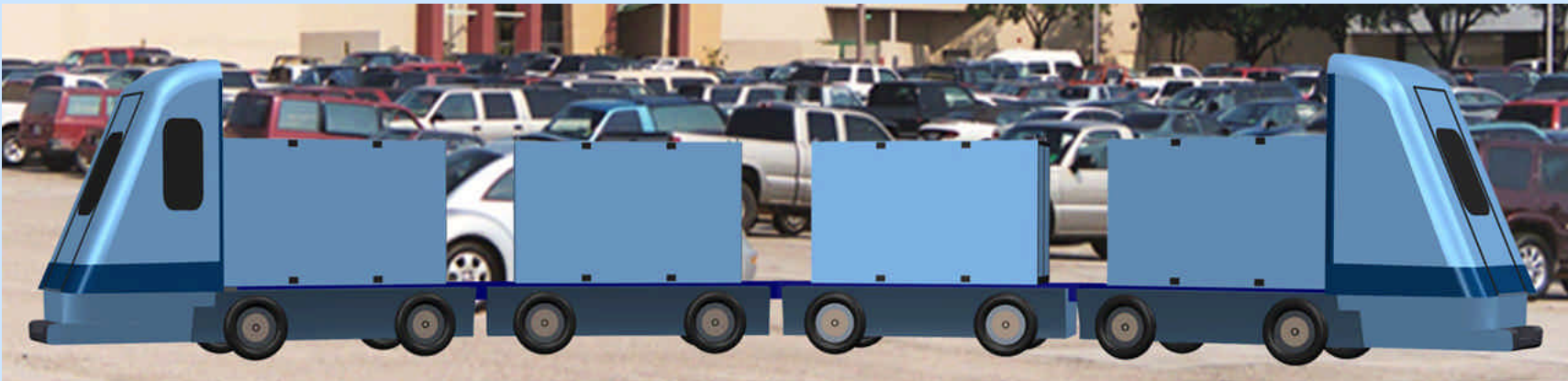
Dualmode cargo tram exits guideway & operates on street in hybrid mode PAT. PENDING
