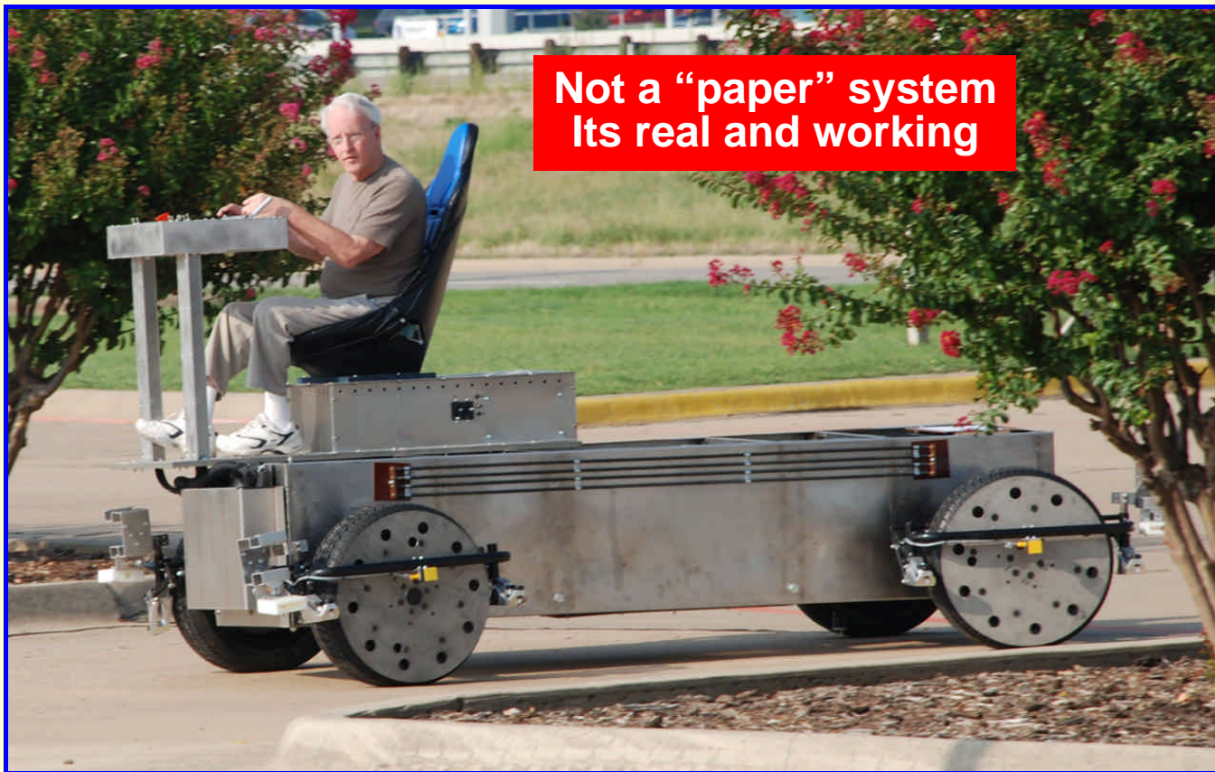
Main chassis unit of hybrid dualmode tram lead car in test ( Dualmode version operates both on guideway & streets )
