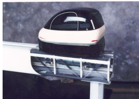
Model PRT Vehicle and Guideway built in Raytheon Model Shop in January 1993 18 months before the fatal decision to go to the configuration shown in Figure 16.
