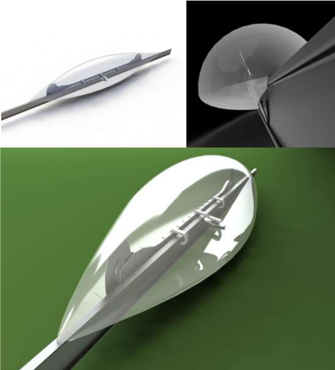
Figure 1 Renderings of feather rail vehicles showing the wheels and fairing. The fairing represents the passenger envelope and can be expanded to allow for more upright sitting position, or lean to increase mileage.
