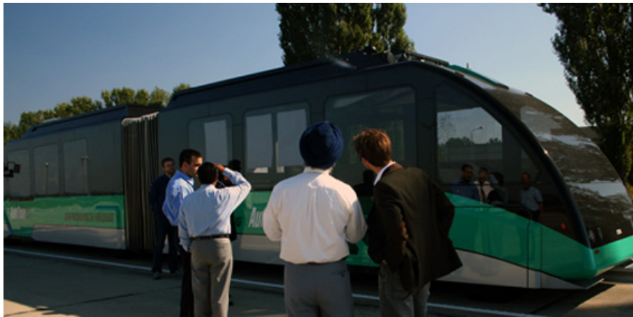
This AutoTram prototype has the same capacity as a large trolley car. Photo courtesy of the Fraunhofer Institute for Transportation and Infrastructure Systems in Dresden.
