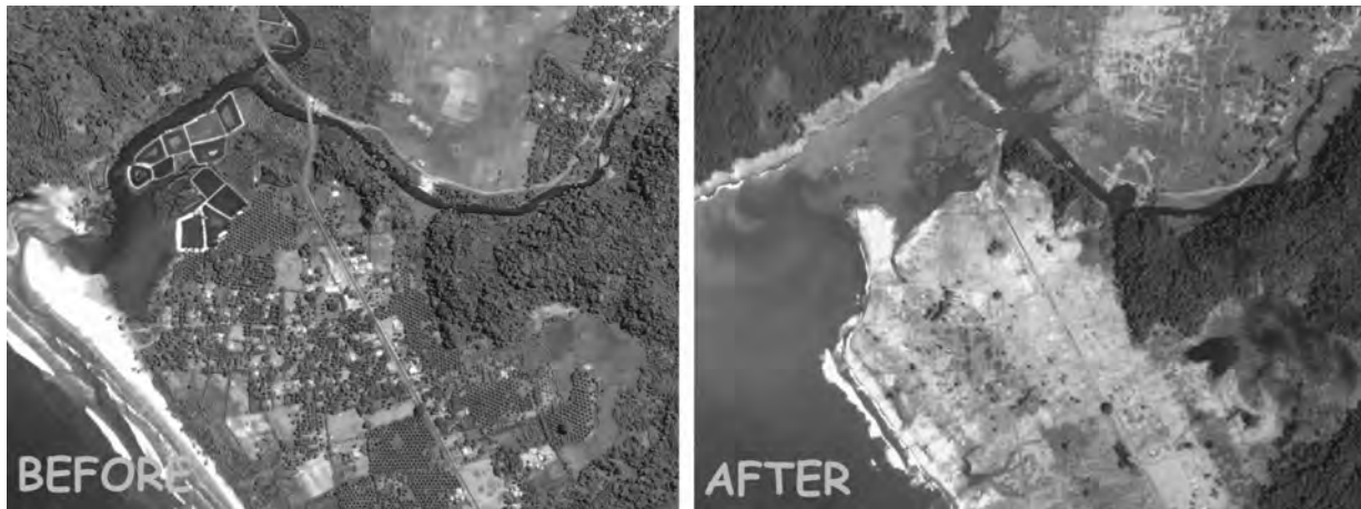
Figure 3.1. Satellite images of Jantang, Aceh (Sumatra, Indonesia) before and after the 26 December 2004 tsunami. Note widening of the river mouth by erosion, stripping of vegetation, and deposition of sand on the coastal plain (light gray color). Images from Digital Globe.
