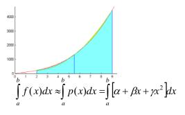
As in the previous (linear) case, the parameters of the interpolant (here  $\alpha$ ,  $\beta$ , and  $\gamma$ ) are expressed in terms of the coordinates  $a, \frac{a+b}{2}, b$  and the value of the function at those points  $f(a), f(\frac{a+b}{2}), f(b)$
