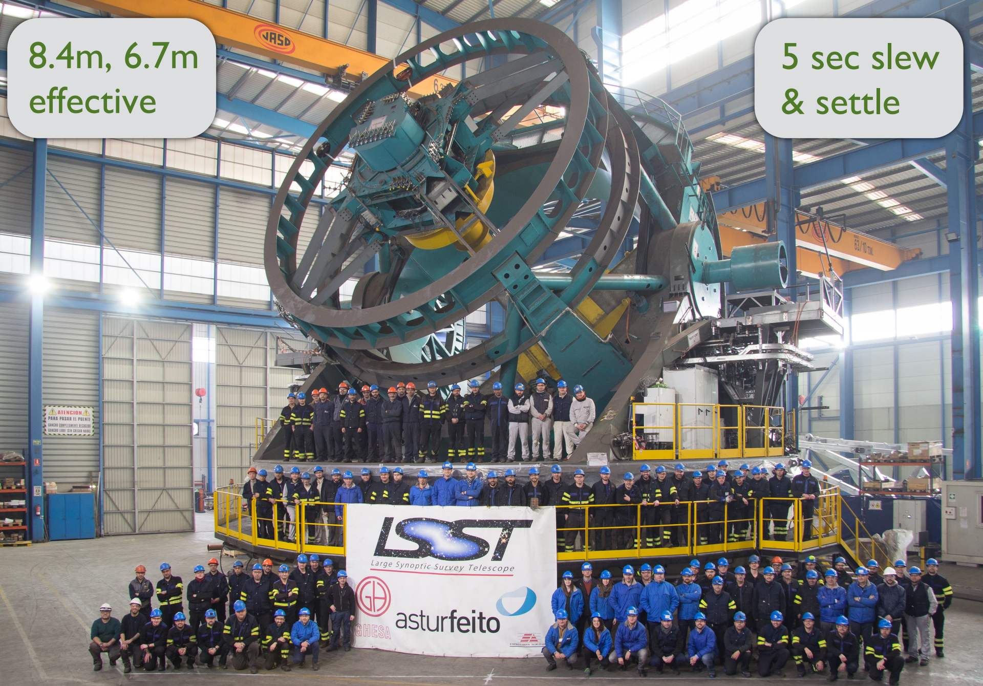
Telescope Mount Assembly before going from Spain to Chile
