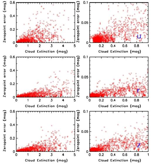
Run 5646, photom. zeropoint error vs. cloud thickness in the urz bands
