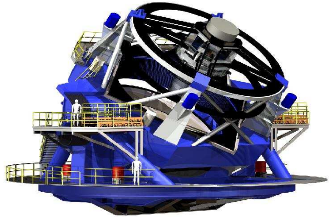
FIG. 8.— The baseline design (modified three-mirror Paul-Baker) for the LSST telescope (current since April 2006).
