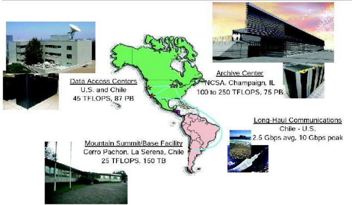
FIG. 17.— The LSST data flow from the mountain summit/base facility in Chile to the data access center and archive centers in the U.S.
