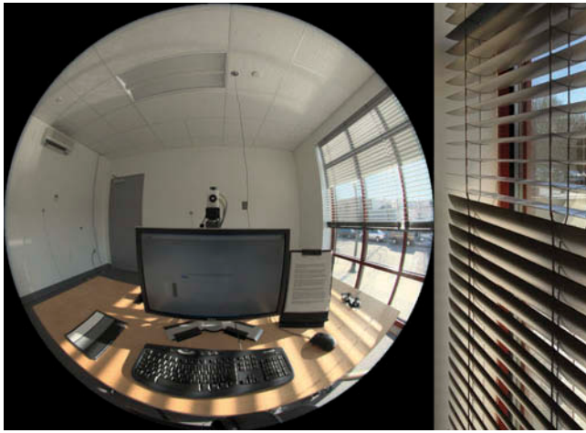
Fig. 1 (left) scene from a participant's point of view; (right) light redirecting blind.
