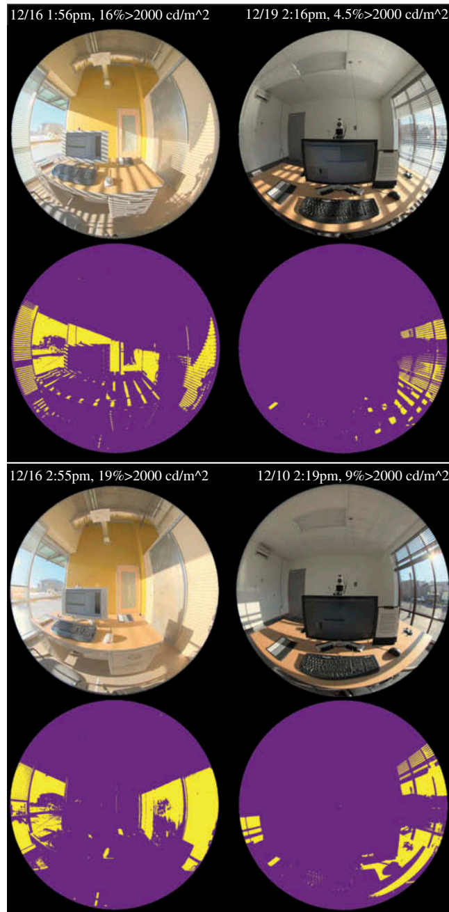
Fig. 11 Similar date- and time-stamped JU scenes; pilot (left), 6-month study (right); yellow > 2000 cd/m 2 .
