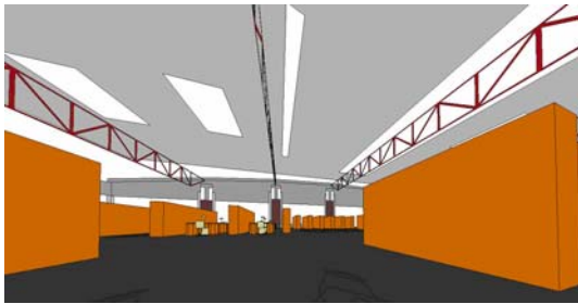
Fig 8. An early design alternative with diffuse skylights
