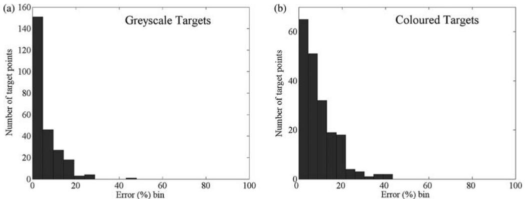
**Figure 10** Histograms for error percentages between the measured and captured luminances for a) greyscale targets; b) coloured targets
