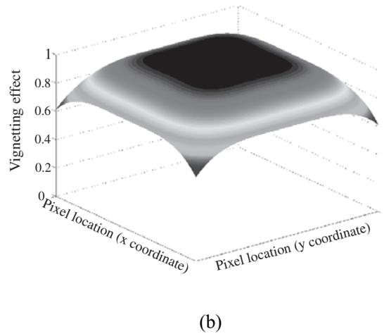
**Figure 8** The vignetting function of Nikon FC9 fisheye lens. a) Measured data points and the vignetting function derived to fit the measured points; b) digital filter developed based on the vignetting function
