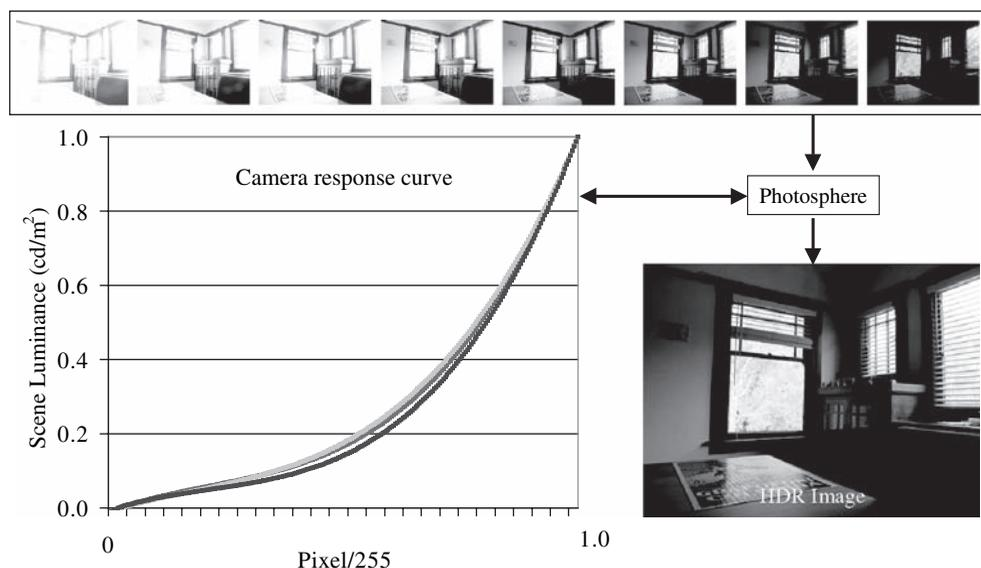
**Figure 1** Camera response curve for Nikon 5400 as determined by Photosphere
