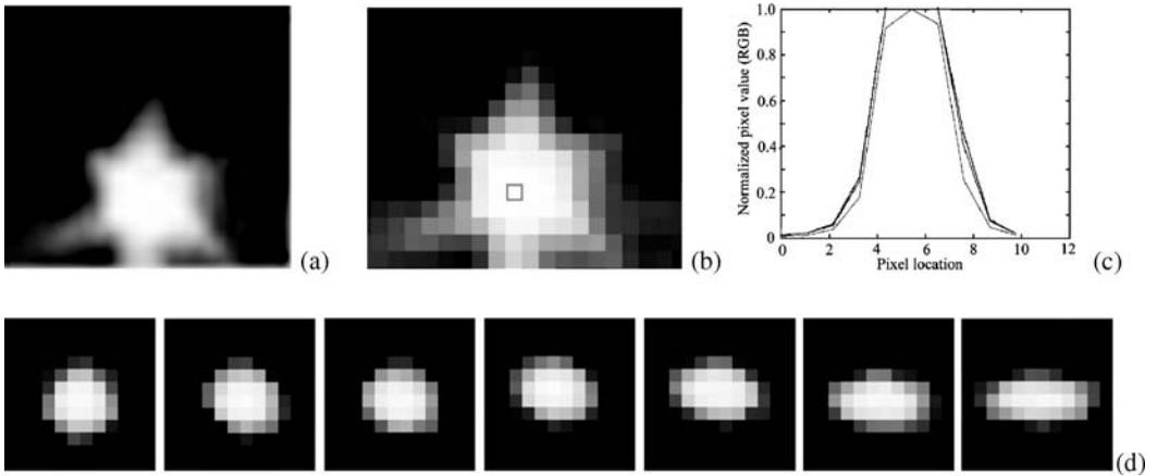
**Figure 9** a) Close-up view of point spreading; the square in (b) shows the pixel that corresponds to the actual light source. c) PSF as quantified from the HDR image; d) PSF as a function of eccentricity (distance from the optical centre) in the camera field of view from 0 to 90° in 15° intervals
