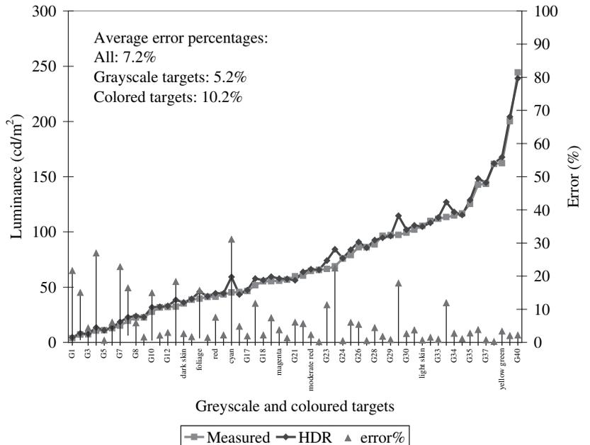
**Figure 5** Coloured and greyscale targets in an office space illuminated with daylighting and electric lighting
