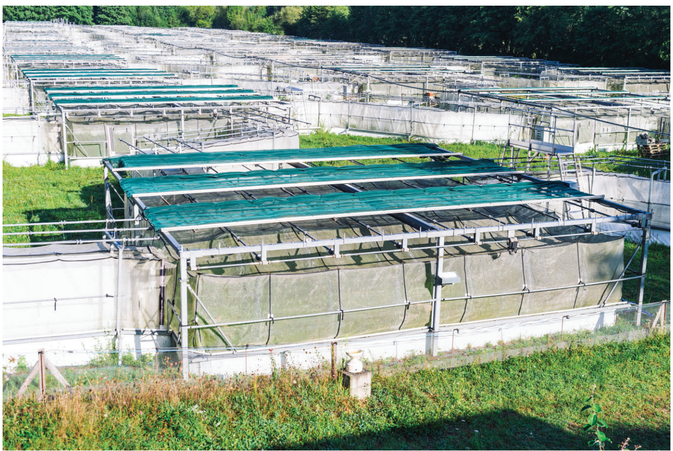
Climate can be manipulated inside population cages of the “métatron,” which is suitable for manipulative studies of responses to seasonal acclimation or to climate (Moulis, France) © Cyril FRESILLON / SETE / CNRS Photothèque
