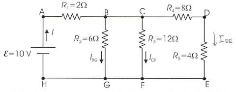
4) [3 points] Compare the magnitude of the current I to  $|I_{BG}+I_{CF}|$  and the magnitude of the potential difference between points EF,  $|V_{EF}|$ , to that between points DE,  $|V_{DE}|$ .
