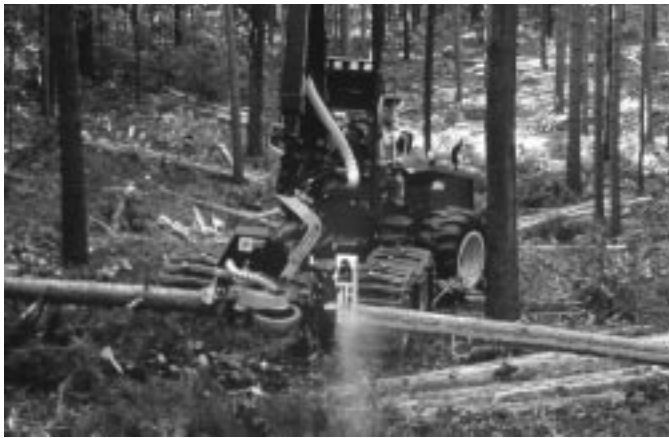
Figure 8 — The typical feller-buncher as used in the Pacific Northwest is track mounted and is designed to work on flat to moderately sloping terrain. Some of these machines have tilting cabs as shown here.
