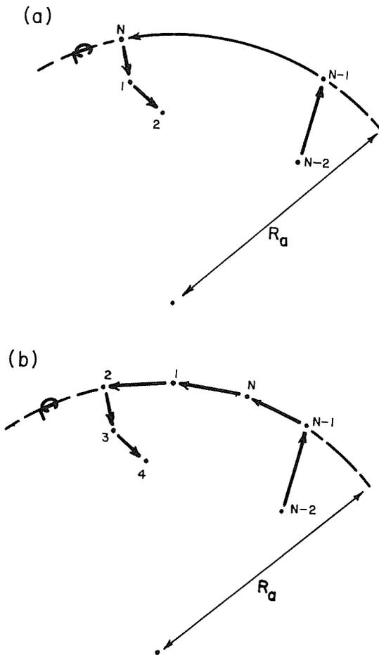
FIG. 5. A region inside a circular curve which is bounded by that curve. That portion of the region defined by the circular curve may be described by either a circular sector (a) or by one or more triangular elements (b).
