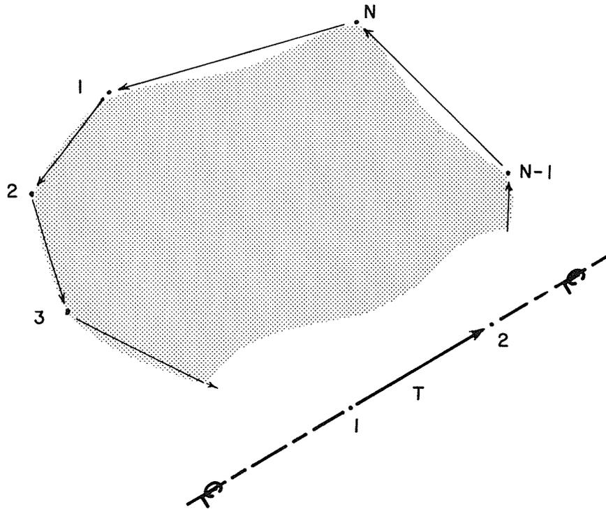
FIG. 1. Plan view of a portion of the cutting unit as delineated by a sequence of directed line segments. The correct orientation of the road center-line tangent vector is also illustrated.
