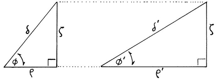
FIG. 3. The ground profiles of the constant slope yarding path before and after the incorporation of a wander factor. Variables associated with profile components are given.
