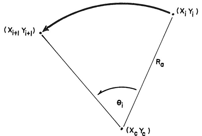
FIG. 4. A circular sector element and associated variables.
