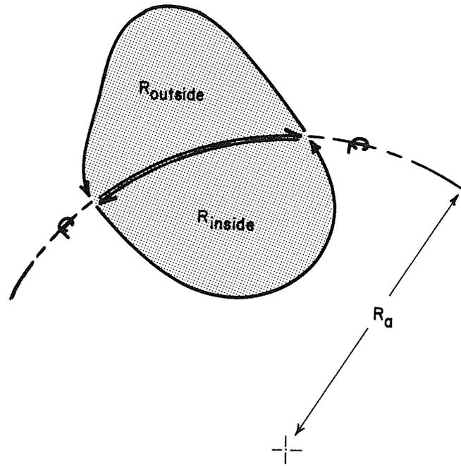
FIG. 2. A cutting unit partitioned into inside and outside regions of the circular curve to which the turns will be yarded.
