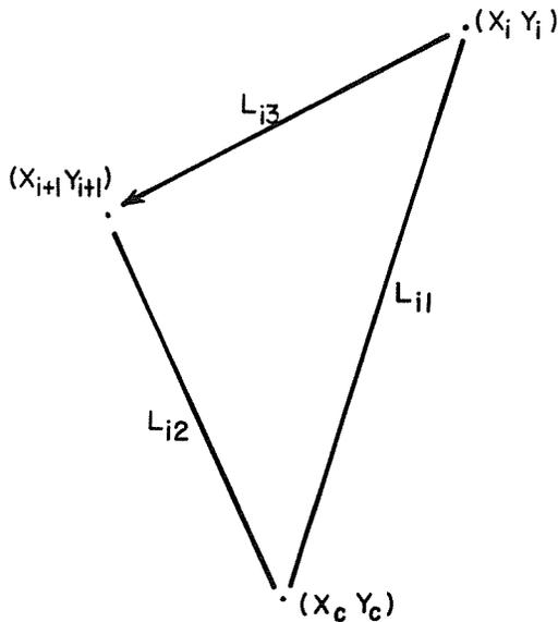
FIG. 3. A triangular element and associated variables.
