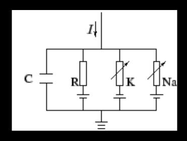
• Then, we set up a differential equation whose parameters we can measure  $CdV/dt=-\Sigma I_{k}(t)+I(t)$
