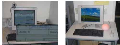
Figure 1: The Ticker and Orb displays used in our studies. left The Ticker, shown in a magnified call-out, is located just above the windows taskbar. right the Orb is the pink globe at the right front of the monitor.
