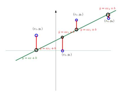
In this picture, the blue circles are the data points, the green line is a candidate for the LMS line, and the black circles are the points on this line aliasing the actual data points. The red segments are the discrepancy between the "theoretical" points  $(x_i, \hat{y}_i = ax_i + b)$  and the true data points  $(x_i, y_i)$ . The line we will choose will be the one that makes the sum of the squares of the lengths of the red segments smallest.
