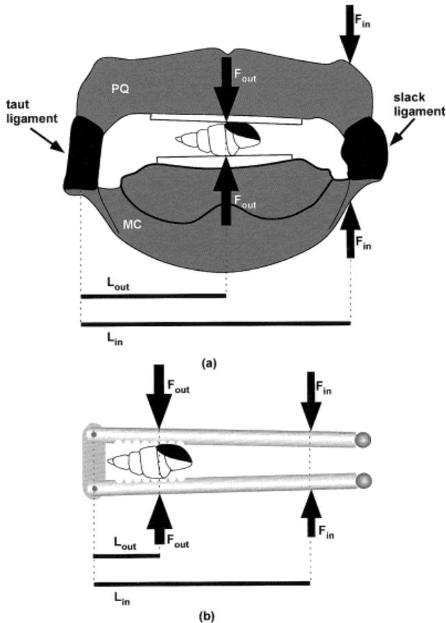
Fig. 9. **a:** The “nutcracker” model of the force advantage of the jaws of the cownose ray, *Rhinoptera bonasus*, in ventral view. A gastropod is shown between the tooth plates, acted upon by a second-class lever powered by the adductors. The ligaments between the upper and lower jaws, shown in black, serve as the fulcrum of the lever system. **b:** A nutcracker of similar proportions showing the principles of the second-order lever system.
