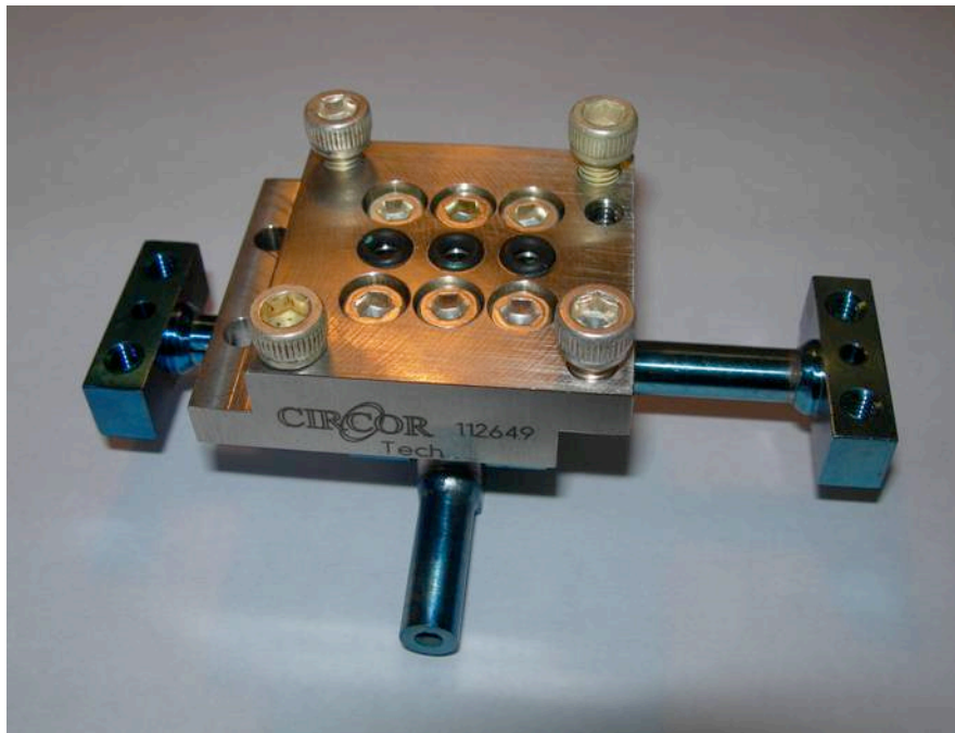
Figure 1 A photograph of the microfluidic mixing device shown without a mixing chamber attached. The two outer black rings are the input pipes and the middle ring is the outlet pipe.
