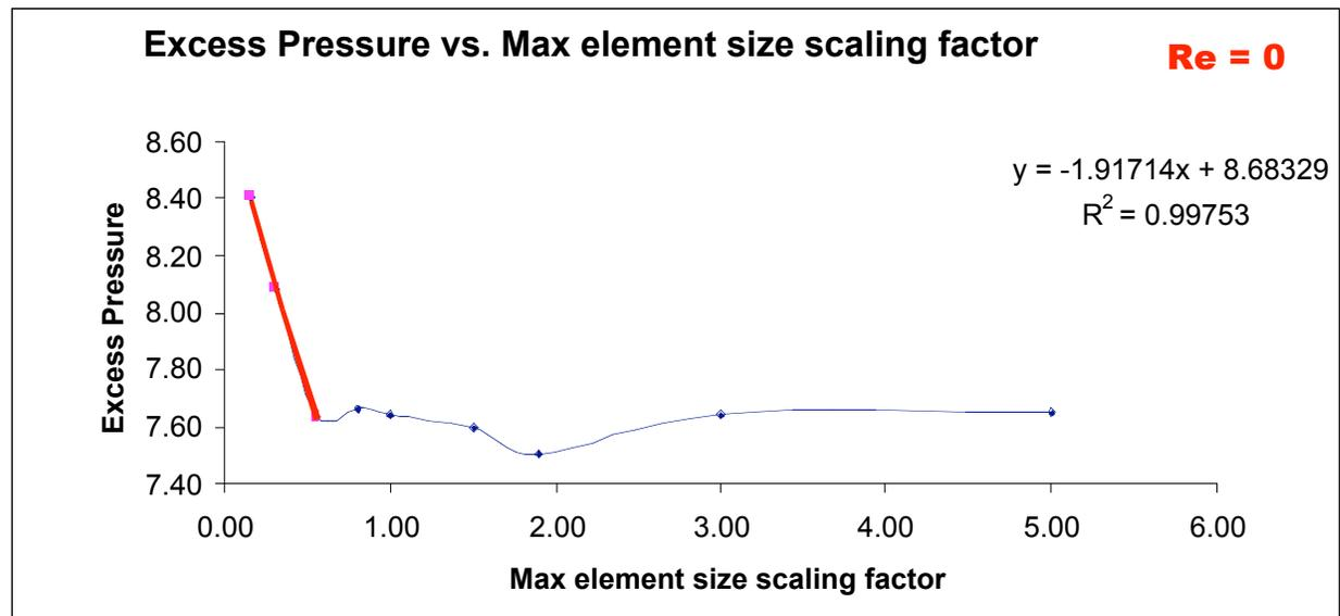
**Figure 2.** Excess pressure drop vs. max element size scaling factor for different mesh refinements for  $Re=0$ .
