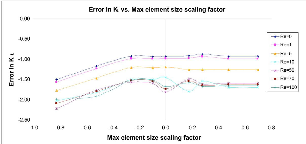
**Figure 5.** Log-log plot of  $K_L$  error vs. mesh size for different  $Re$  values.
