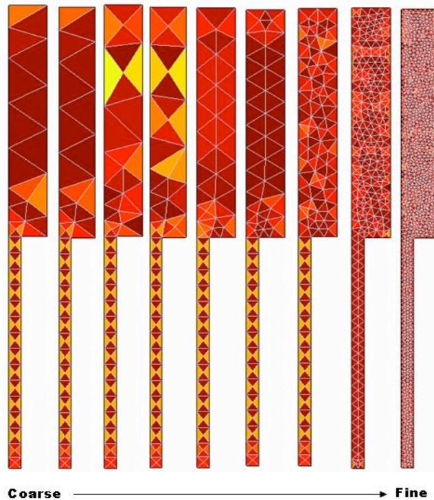
**Figure 1.** *Spectrum of mesh refinement presets in COSMOL Multiphysics software.*
