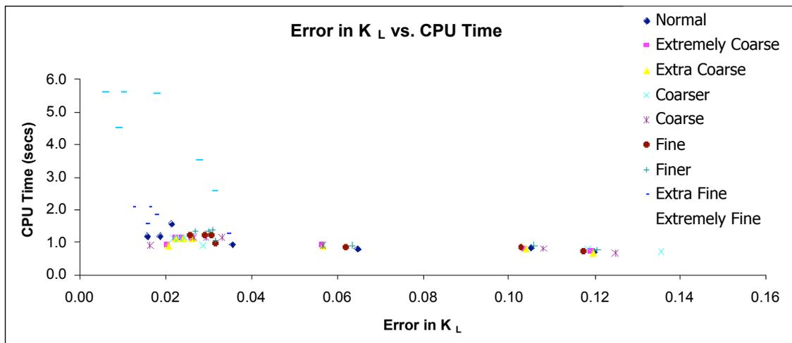
**Figure 4.**  $K_L$  error vs. CPU time for different mesh refinement presets.
