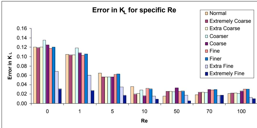
**Figure 3.**  $K_L$  error distribution for different Reynolds numbers and refinement presets.
