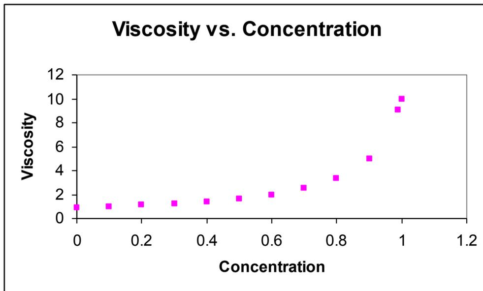
Figure 2: Proposed model for the Viscosity as function of Concentration for the solid in the well.
