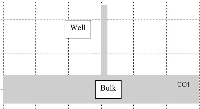
Figure 2: The basic etching Model. The pore is modeled as a well with an aspect ratio of 10:1 (length:width).
