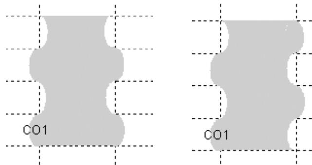
Figure 1a. Symmetric Pore Waviness. Figure 1b. More realistic representation of the uneven pore waviness.
