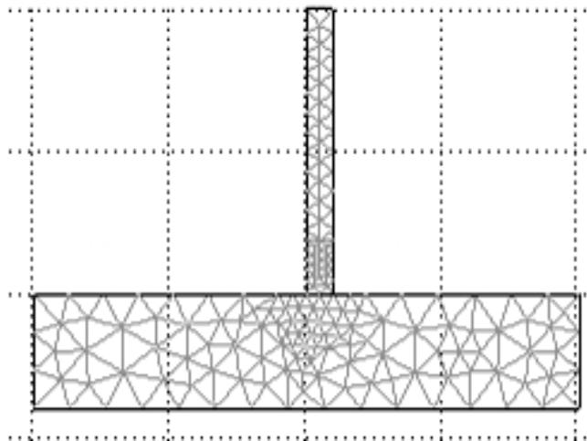
Figure 6: Mesh for the Etching Diffusion file. The boundaries and subdomain are the same as the previous file.
