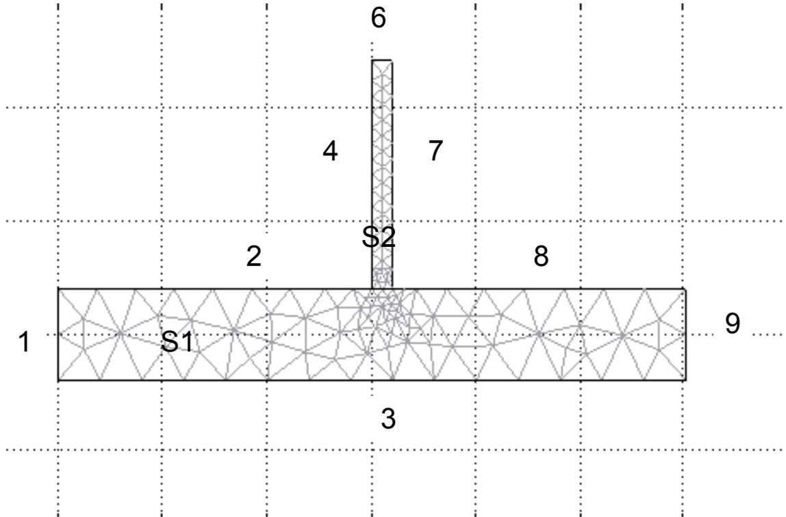
Figure 4: Mesh for the Etching Reaction file and the boundary/subdomain specifications. The mesh was refined only around the pore opening.
