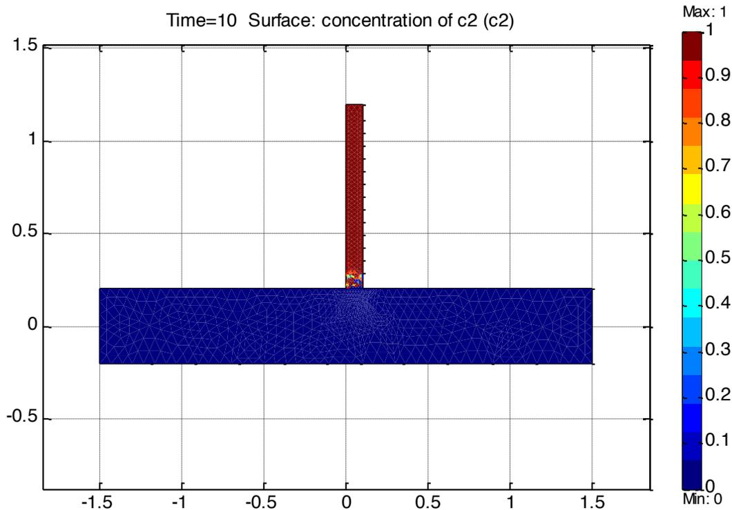
Figure 5: Etching Reaction results for  $t=10$ .
