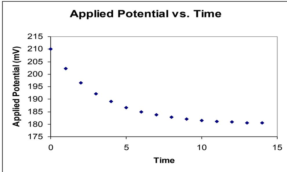
Figure 3: Applied potential versus time for the electrochemical portion of the dissolution reaction.
