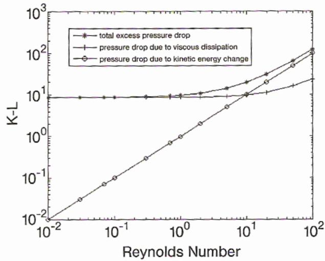
Fig. 8.4 Laminar flow excess pressure drop for a 3 : 1 contraction in a circular channel.  $K_L$  is the total pressure minus the fully developed pressure drop in the two regions, expressed as  $K_L = \Delta p_{\text{excess}} d_2 / \eta \langle v_2 \rangle$ .
