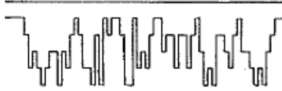
Figure 1: Section of the channel containing random ridges on one plate 1 . Figure is scaled by a factor of four in the vertical direction.
