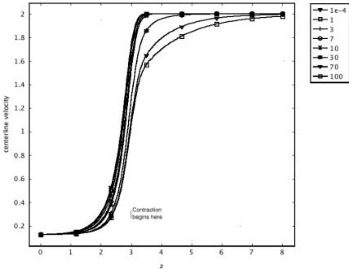
Figure 8. Velocity rearrangement before contraction, 4:1 contraction, cylindrical geometry for different Reynolds numbers based on the downstream section
