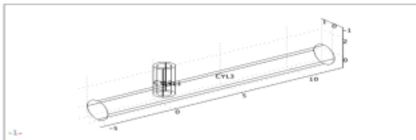
**Figure 20. Reactor with two inlets for two reagents and a catalyst**
