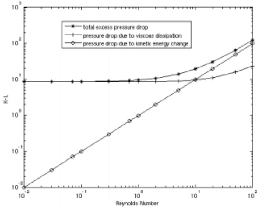
**Figure 4. Laminar flow excess pressure drop for a 3:1 contraction in a circular channel.**
