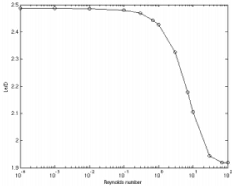
Figure 9. Approach length, 5% criterion, 4:1 contraction, cylindrical geometry
