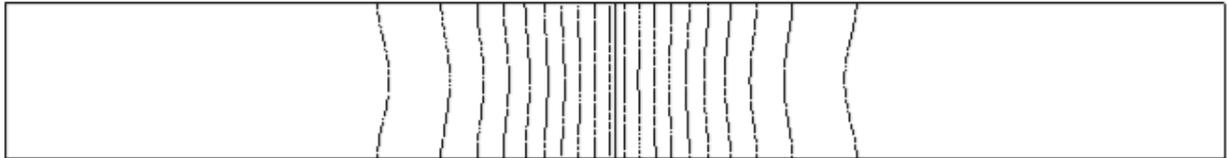
(b) Concentration at exit with velocity profile allowing slip on the side walls, for the same average velocity as (a); variance = 0.195
