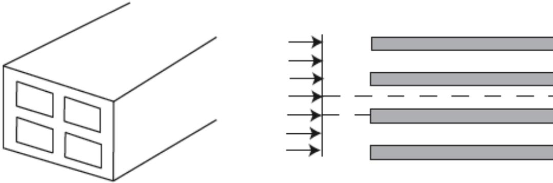
**Figure 5. Manifold with square holes (left) or flat plates (right)**
