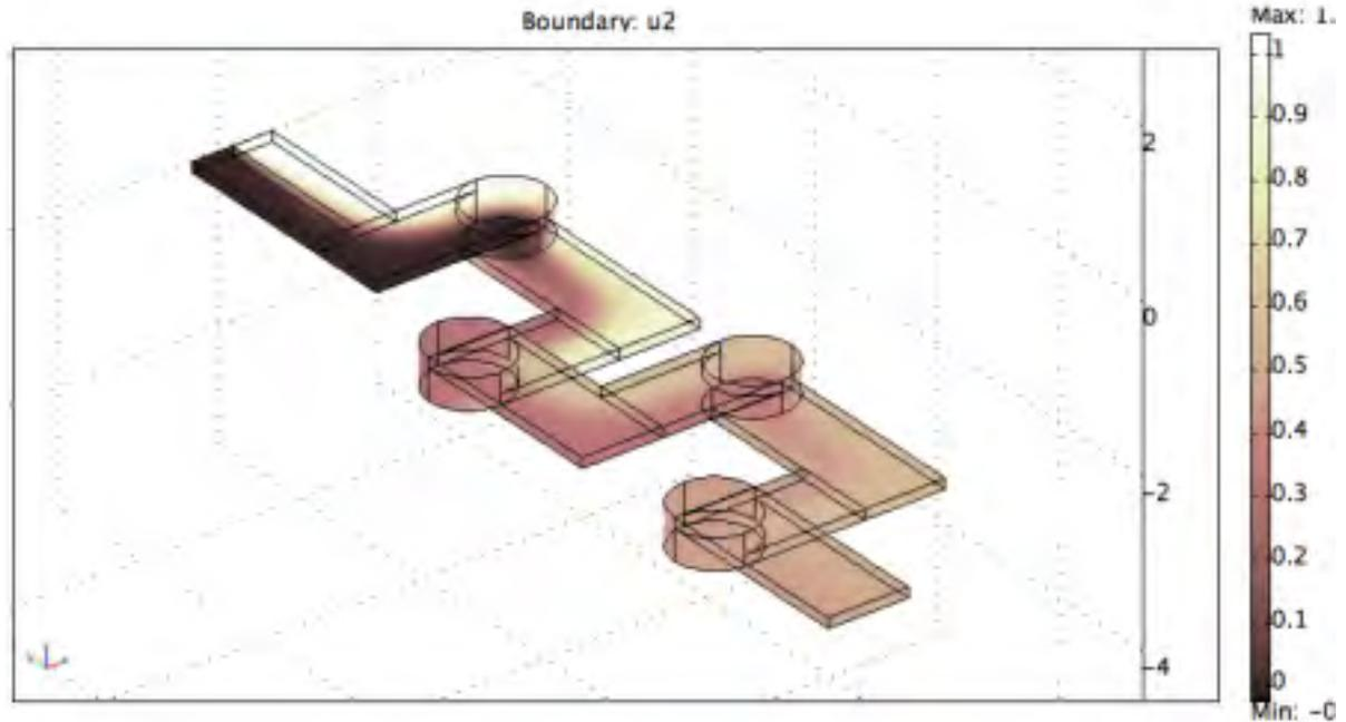
**Figure 19. Concentration on surface of the serpentine mixer;  $Re = 1$ ,  $Pe = 1000$ ,**
