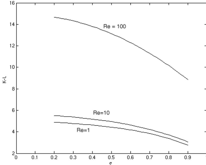
Figure 7.  $K_L$  defined by Eq. (14) for various planar contractions for a manifold; the curve for  $Re = 0$  is indistinguishable from that for  $Re = 1$ .
