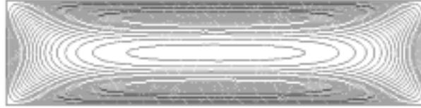
**Figure 12a. Fully developed velocity profile in a 1 x 4 rectangular channel**
