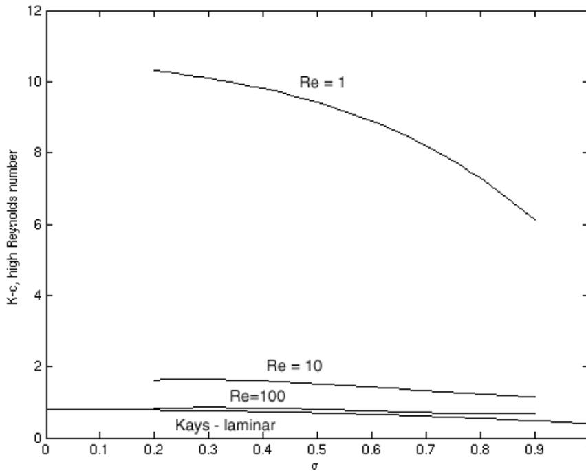
Figure 6.  $K_c$  defined by Eq. (18) for various planar contractions for a manifold
