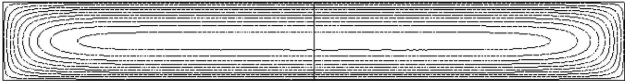
**Figure 12b. Fully developed velocity profile in a 1 x 8 rectangular channel,
