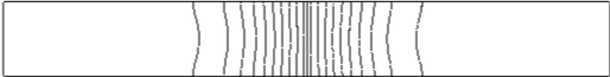
(a) Concentration at exit with fully developed velocity profile; variance = 0.193
