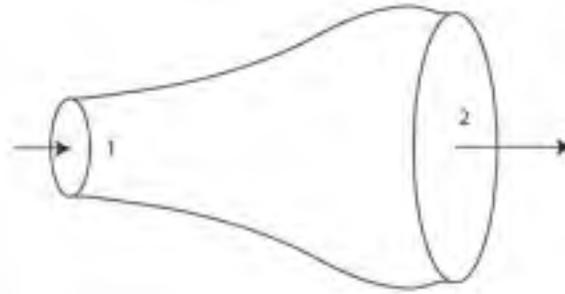
**Figure 2. Geometry and notation for mechanical energy balance**
