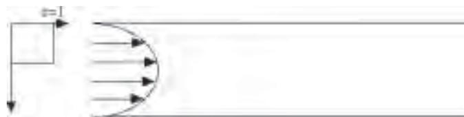
**Figure 11. Diffusion in fully developed planar flow**
