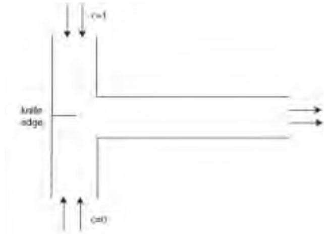
**Figure 16. T-sensor; the knife edge can be added as shown**
