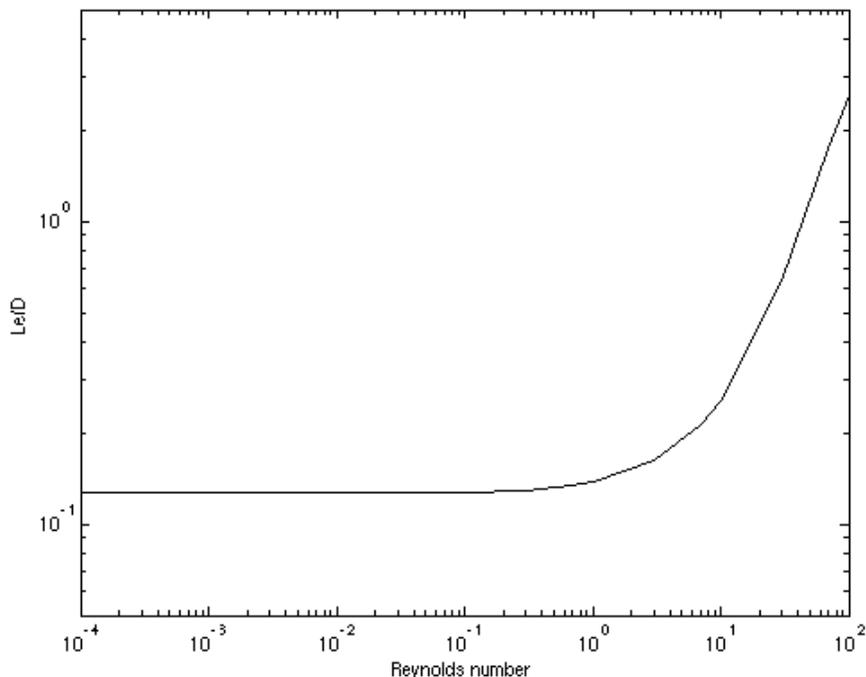
**Figure 10. Entry length, 5% criterion, 4:1 contraction, cylindrical geometry**
