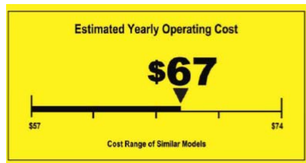
FIGURE 2. PORTION OF THE ENERGYGUIDE LABEL SHOWING A CONTINUOUS SCALE AND SPECIFIC VALUE FOR YEARLY ENERGY COST.
