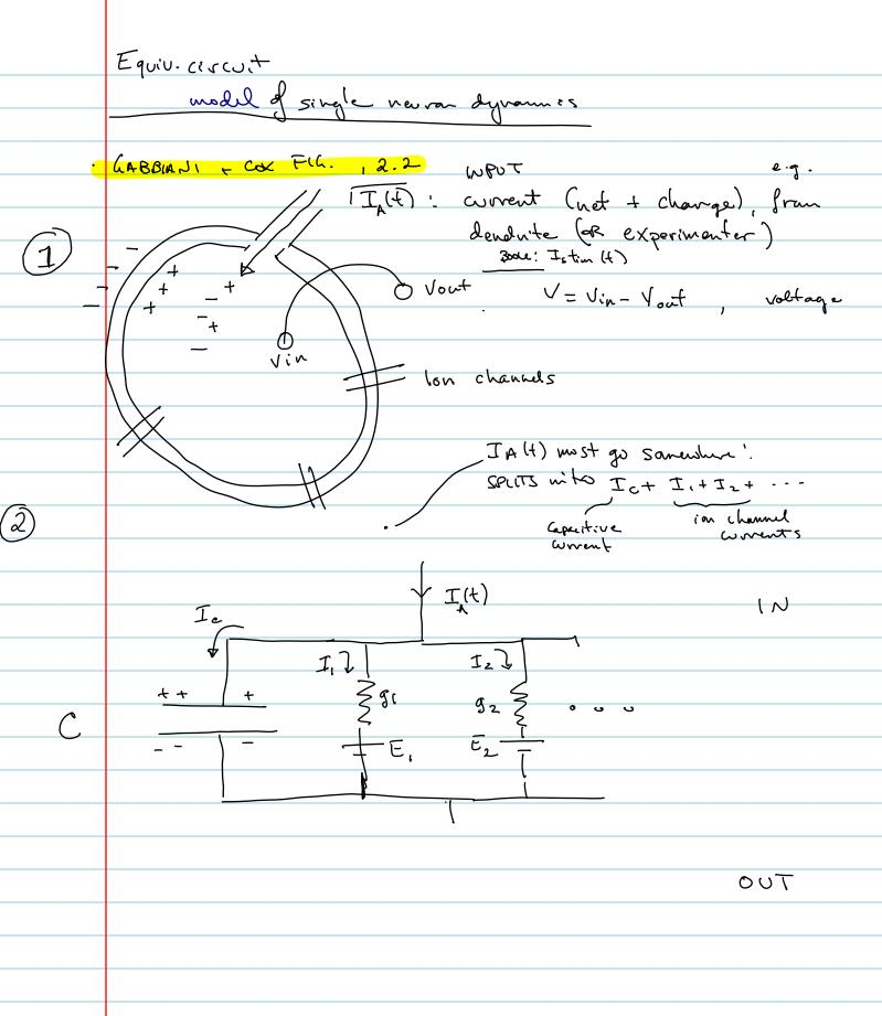
CAPACHTOR: Q = CV Q: Change on "top" wall / plat e C: capacitance # = IC Corrent: Change in charge / Unit  $\Rightarrow T_{c} = \frac{d}{dt}(CY) = c\frac{dV}{dt}$ (5.2, A+D) OHN'S LAND
