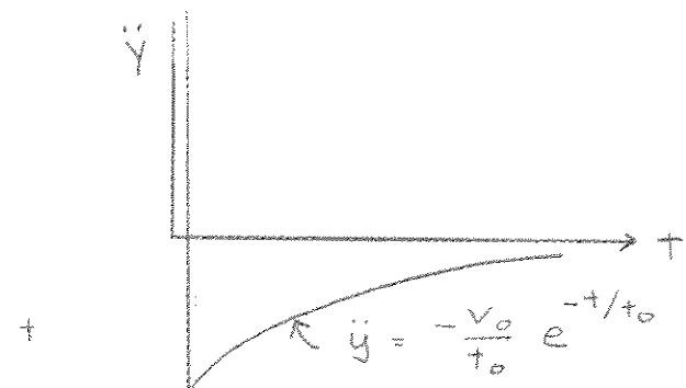
To instantaneously go from an initial velocity = 0 to  $\dot{y} = V_0$  requires  $\ddot{y}(0) = \infty$ . But since the velocity is not infinite, the integral of the acceleration must be finite.
