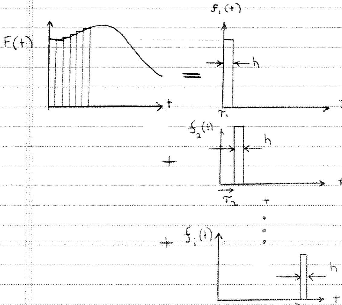
Obtain the solution  $u_i(t)$  for the driving force  $f_i(t)$ , where  $f_i(t)$  is a block pulse of length  $h$  which begins at  $t = \tau_i$ .
