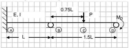
**Problem 1.** Consider this structure as THREE BEAM MEMBERS (AB, BC and CD), with joint loads and moments (no member loads). Solve this problem by implementing the direct stiffness method using a spreadsheet, as shown in class. You may work in groups of two to prepare the spreadsheet for Problem 1. List your spreadsheet partner on the first page of your solution. Complete other parts of your Problem 1 (e.g., load, shear and bending moment diagrams) individually.
