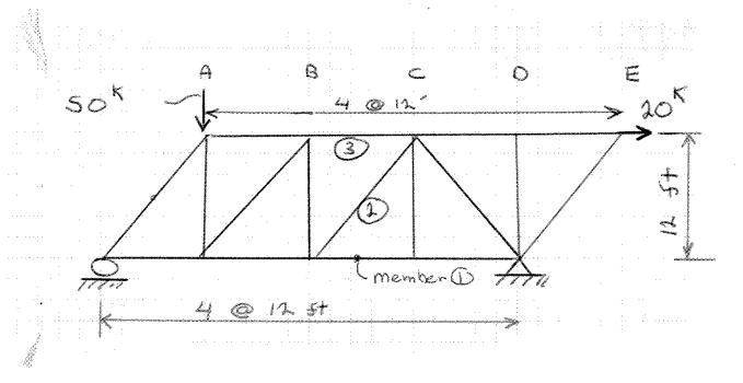
Problem 4 (30) The 2D truss system shown below is subjected to an applied force.
