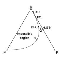
Any set of three numbers summing to 1 can be represented as a point in a unit-height triangle.
