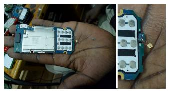
Figure 2: The discarded microphone is visible on Jason's palm. He has connected a replacement microphone using four copper wires, rather than mounting it on the motherboard, as can be seen in the magnified image, September, 2012.
