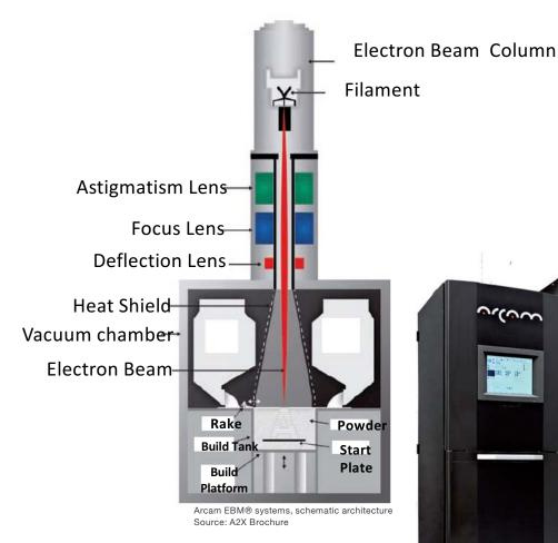
ARCAM® A2X EBM Additive Manufacturing Machine
