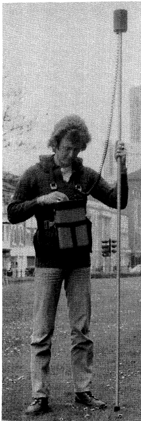
Proton magnetometer and map of a magnetic survey on a site in the Derbyshire coalfield. Stations are on 3 m grid; contours are at 100 nT intervals above a base of 48 000 nT. Dipole anomalies lie over one known shaft and indicate the location of two more shafts
