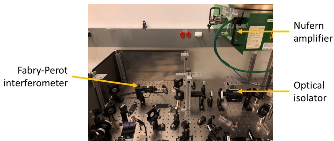
Figure 4.11: A photo of the Nufern amplifier and the optics at its output.
