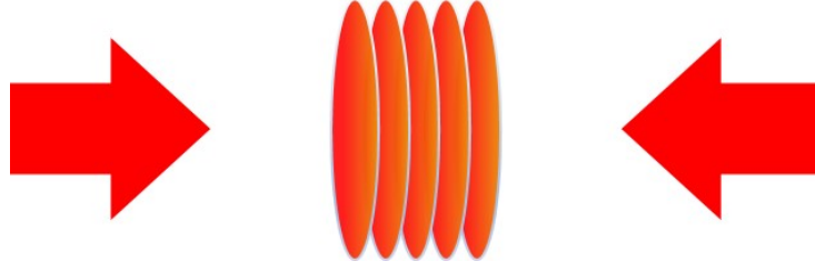
Figure 3.3: One-dimensional optical lattice. A one-dimensional optical lattice is formed by overlapping two linearly-polarized laser beams propagating in opposite directions. The resulting optical potential is a stack of 2D pancake-like traps.
