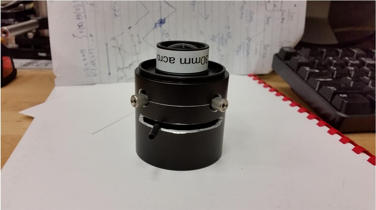
Figure 2.14: The slightly anthropomorphic iris translation stage mounted in a 2" lens tube, via some band saw modifications to the lens tube. This contraption is part of the readout light collection optics.
