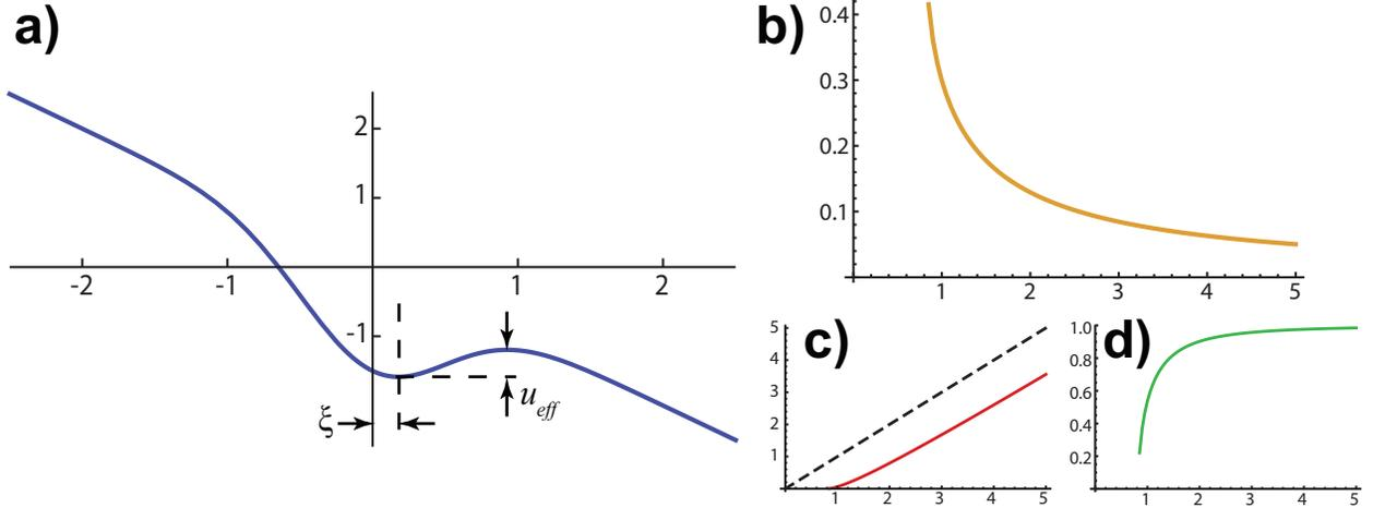
Figure 8.7: Properties of the tilted trap, computed using numerical software, and plotted vs the reduced nominal trap depth  $u_0$ . a) Schematic of the tilted Gaussian 1D potential. b) Displacement  $\xi$  of the trap minimum from the center of the ODT beam. (I.e. sag distance) c) Effective trap depth  $u_{eff}$ . The dashed line shows the nominal trap depth  $u_0$  for comparison. d) Modified trap frequency, in units of the frequency of an un-tilted trap of equal depth and waist.
