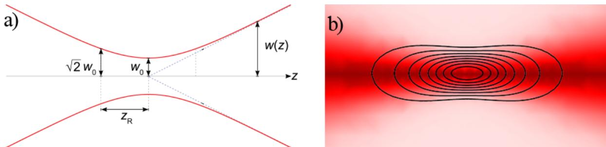
Figure 8.1: A lowest-transverse-order ( $\text{TEM}_{0,0}$ ) Gaussian laser beam. a) Geometry of beam, showing the hyperbolic form of the beam near the focus. Beam waist  $w_0$ , beam width  $w(z)$ , and Rayleigh length  $z_R$  are shown. b) Intensity distribution of beam near focus, with equipotential lines.
