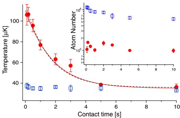
FIG. 2 (color online). Sympathetic cooling of  ${}^6\text{Li}$  (red solid circles) by thermalization with a cold  ${}^{174}\text{Yb}$  bath (blue open squares). The temperatures equilibrate with an exponential time constant of  $(1.7 \pm 0.2) \text{ s}$  (black dashed line). The red solid line is the result of a numerical model (see text). The inset shows the numbers of the two species which are almost an order of magnitude apart.
