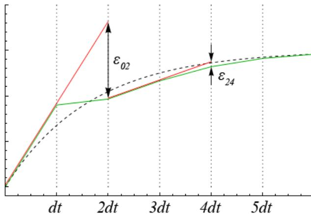
Figure 13.6: Numerical solution to a dynamical system (green line) together with the exact solution (black, dashed line). The red lines are extrapolations of the green line segments, used to estimate  $\epsilon_{i(i+2)}$ , the reduction in error from step size  $2\Delta t$  to step size  $\Delta t$ . Depending on the desired tolerance, the first two steps may require further bifurcation, whereas steps 3-4 may not.
