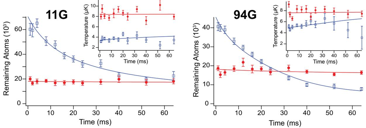
Figure 15.3: Population dynamics of simultaneously trapped  $\text{Yb}^* m_J = -1$  and Li in its absolute ground state. Insets show the temperature evolution, and solid lines are best-fits to a theoretical model.
