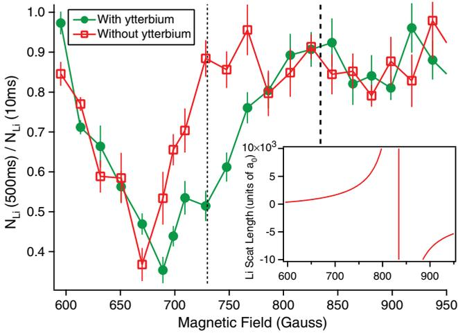
FIG. 1. (Color online) Li atom-loss spectroscopy in the presence (filled circles) and absence (open squares) of a Yb bath near the  $^6\text{Li}$  834 G Feshbach resonance (inset). We plot the number of Li atoms after 500 ms of evolution normalized to that at 10 ms. The thick dashed line indicates the resonance center and the thin dashed line indicates the magnetic field at which  $\epsilon_B = k_B T_{\text{Li}}$  for the initial conditions.
