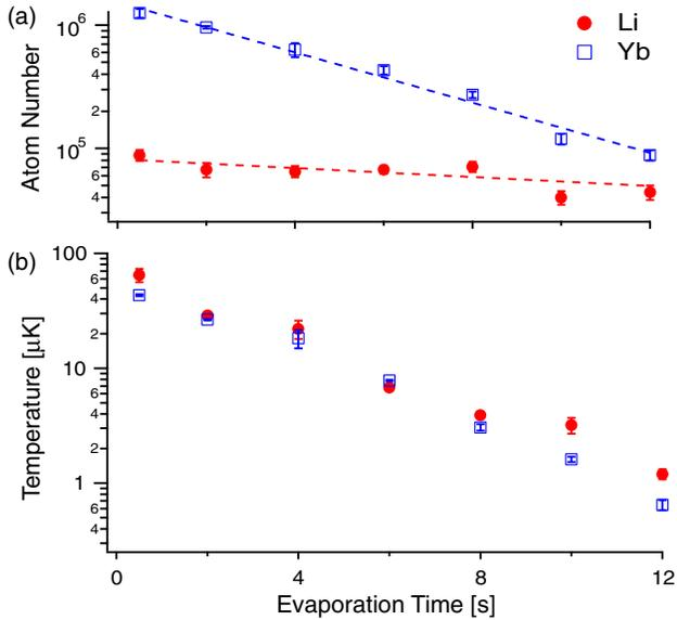
FIG. 3 (color online). Sympathetic cooling of lithium by forced evaporative cooling of ytterbium. (a) Number and (b) temperature evolution for <sup>6</sup>Li (solid circles) and <sup>174</sup>Yb (open squares) as the power in the crossed optical dipole trap is reduced by a factor of 28 over 12 s, corresponding to an approximately exponential ramp with a time constant of 2.9 s.
