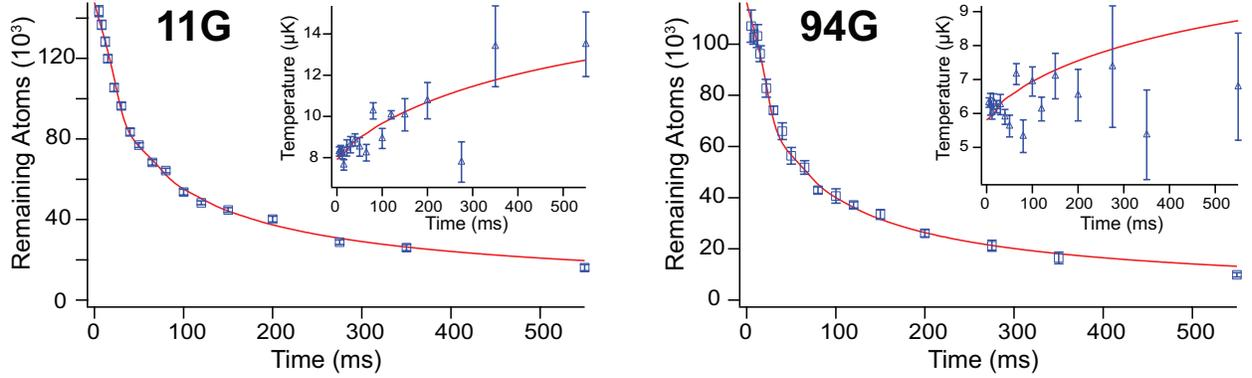
Figure 15.2: Population dynamics of  $\text{Yb}^*$  in the  $m_J = -1$  state. Measurements are performed at two magnetic fields. Insets show the temperature evolution, and solid lines are best-fits to a theoretical model.
