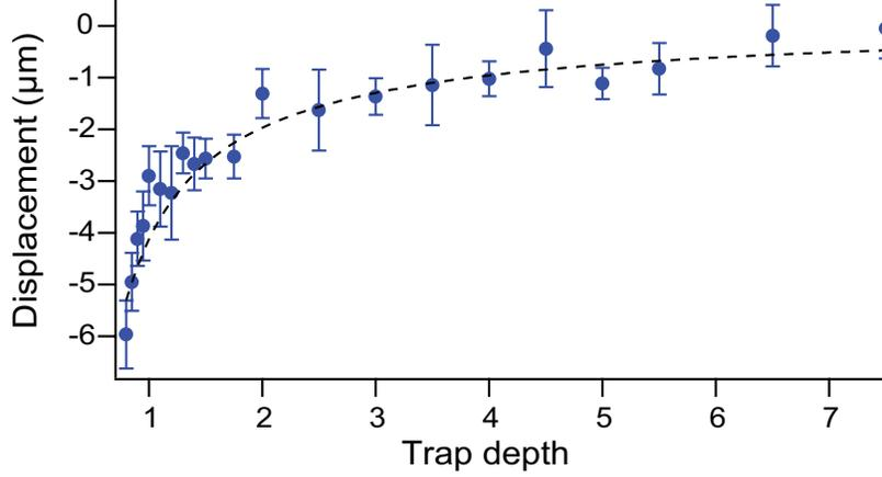
Figure 14.1: Ytterbium sag data for a range of trap depths. The x-axis is the analog control voltage  $V_{contr}$ , which is proportional to the trap depth. The dashed line is a best-fit of the model function  $y(V_{contr}) = y_0 + w_0 \times \xi(V_{contr}/V_0)$ , with  $V_0$  constrained by equation (14.12).
