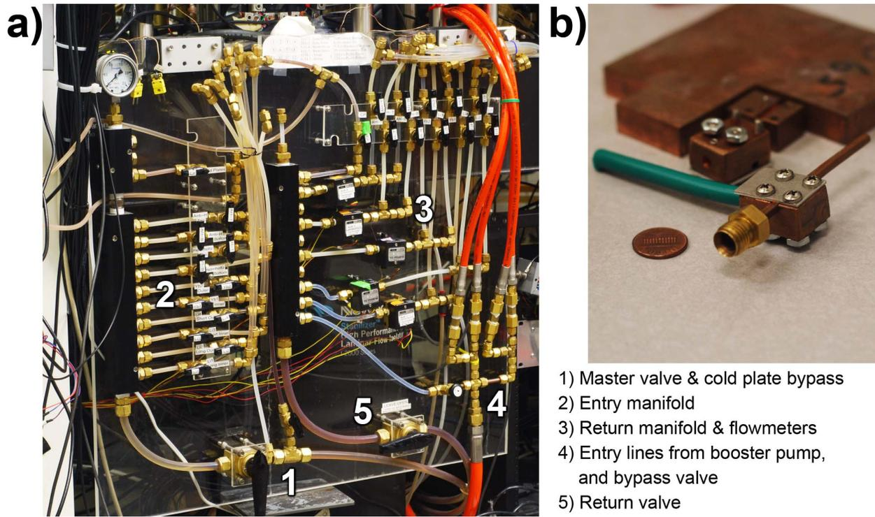
Figure 6.4: a) Photograph of water distribution panel. b) Photograph of a square wire interface. The compression fitting cap has been equipped with a square hole, and is brazed onto the square wire.
