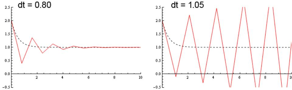
Figure 13.5: Solutions to the differential equation  $y' + 2y - 2 = 0$ ,  $y(0) = 2$ , using the forward-Euler method, (red lines) shown together with the analytic solution (dashed line). If the step size of the iteration is chosen to be appropriately small the Euler method rapidly converges to the true steady-state solution. If the step size is too large, the numerical solution diverges.
