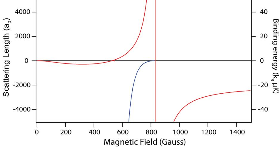
Figure 2.4: The  ${}^6\text{Li}$  Feshbach resonance at 834G. By tuning the magnetic field, one may access a wide range of interactions, (red line) from strongly repulsive ( $a \gg 0$ ) to strongly attractive ( $a \ll 0$ ), as well as interaction-free regions at the zero-crossing at 528G. A bound state of the  $\text{Li}_2$  molecule (blue line) dissolves into the free-particle continuum at the resonance point, giving rise to the divergent scattering behavior.
