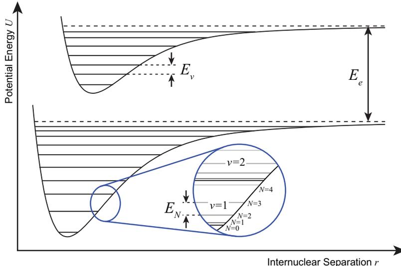
Figure 3.1: Schematic of rotational, vibrational and electronic structure. The vibrational and rotational level splittings,  $E_v$  and  $E_N$  have been greatly exaggerated for clarity. A molecular potential typically has  $\mathcal{O}(100)$  vibrational levels, each with a manifold of rotational sublevels.
