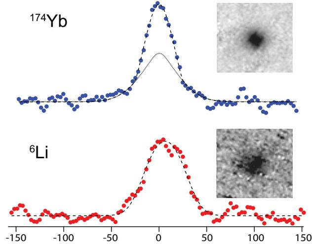
Figure 12.1: Density traces of simultaneously degenerate (bosonic) ytterbium and (fermionic) lithium. Atom numbers are  $2.3(1.2) \times 10^4$  for Yb(Li), with reduced temperatures  $T/T_C = 0.8$ ,  $T/T_F = 0.3$ , respectively. The insets are cropped sections from the absorption images from which the data was extracted.
