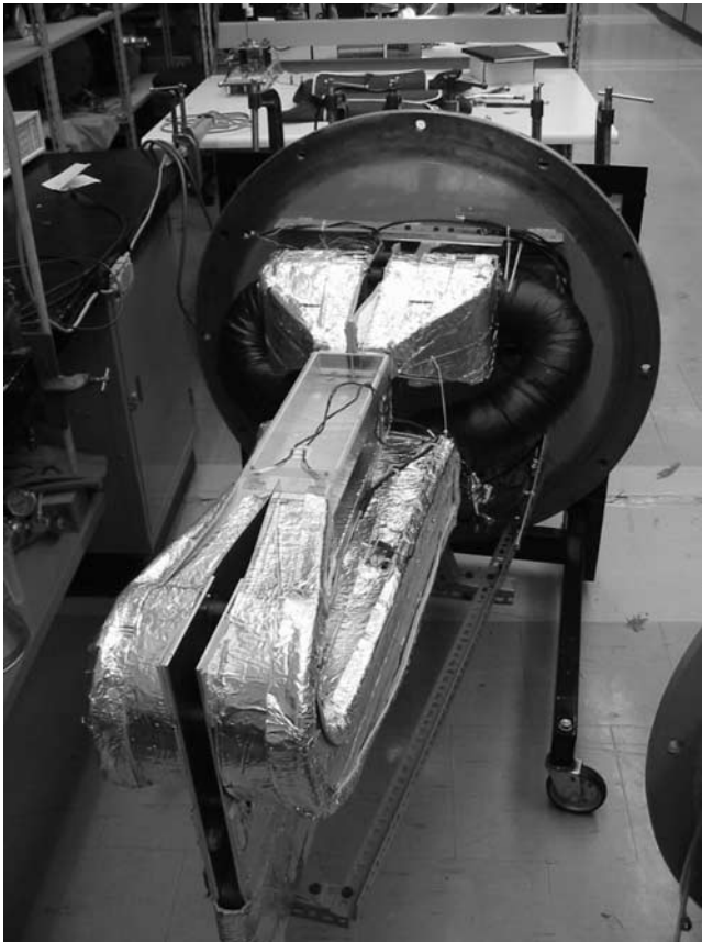
Figure 3a. The calibration tunnel mounted on the door of the Mars chamber. The test section (top, middle) shown here is the one used for solar heating effects.
