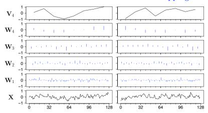
$\bullet$  Haar DWT of FD(0.45) series **X** (left-hand column) and level j=3 tree-based bootstrap thereof (right-hand)
